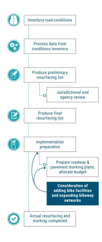
FIGURE 1: Typical approach to identifying and preparing projects for resurfacing
