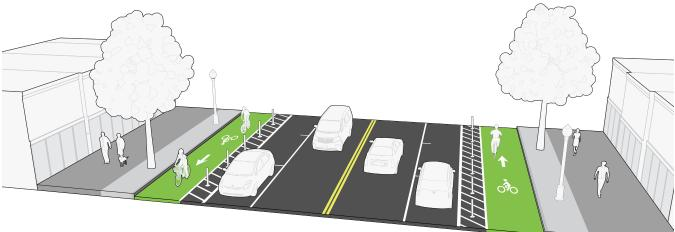
FIGURE 11: Sample illustration of a street after a four to two Road Diet and the installation of separated bike lanes.
