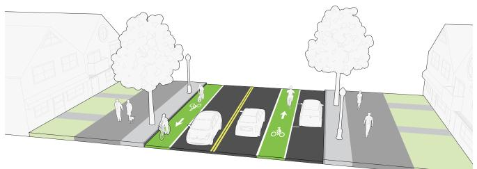
FIGURE 13: Sample illustration of a street after parking removal on one side to include bike lanes.
