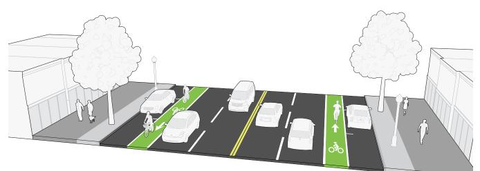
FIGURE 5: Sample illustration of a street after a Lane Diet and the installation of bike lanes.
