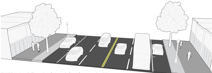
FIGURE 10: Sample illustration of a street before a four to two Road Diet.
