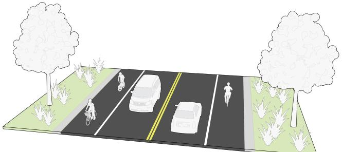
FIGURE 16: Sample illustration of a road after having the shoulders paved.
